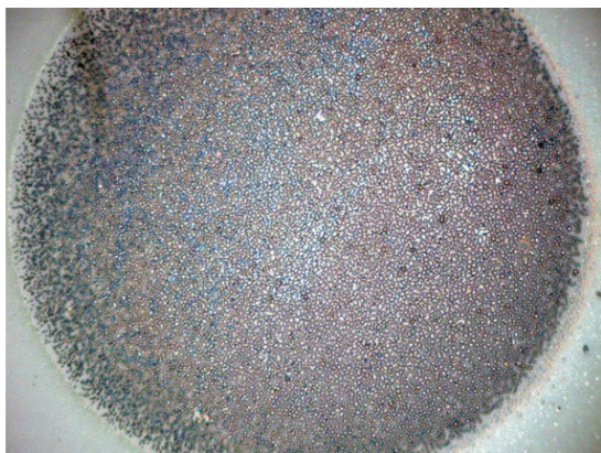
Fig. 2. Microarray cell after colorimetric detection based on the enzymatic oxidation of o -dianisidine and 4-chloro-1-naphthol (the photograph was made on an Axio Imager A1m optical microscope (Carl Zeiss)).
